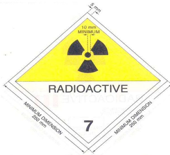
Figure 6. Placard. Minimum dimensions shall be as shown; when different dimensions are used the relative proportions must be maintained. The number '7' shall not be less than 25 millimeters high. The background colour of the upper half of the placard shall be yellow and of the lower half white, the colour of the trefoil and the printing shall be black. The use of the word "RADIOACTIVE" in bottom half is optional to allow the alternative use of this placard to display the appropriate United Nations for the consignment.
